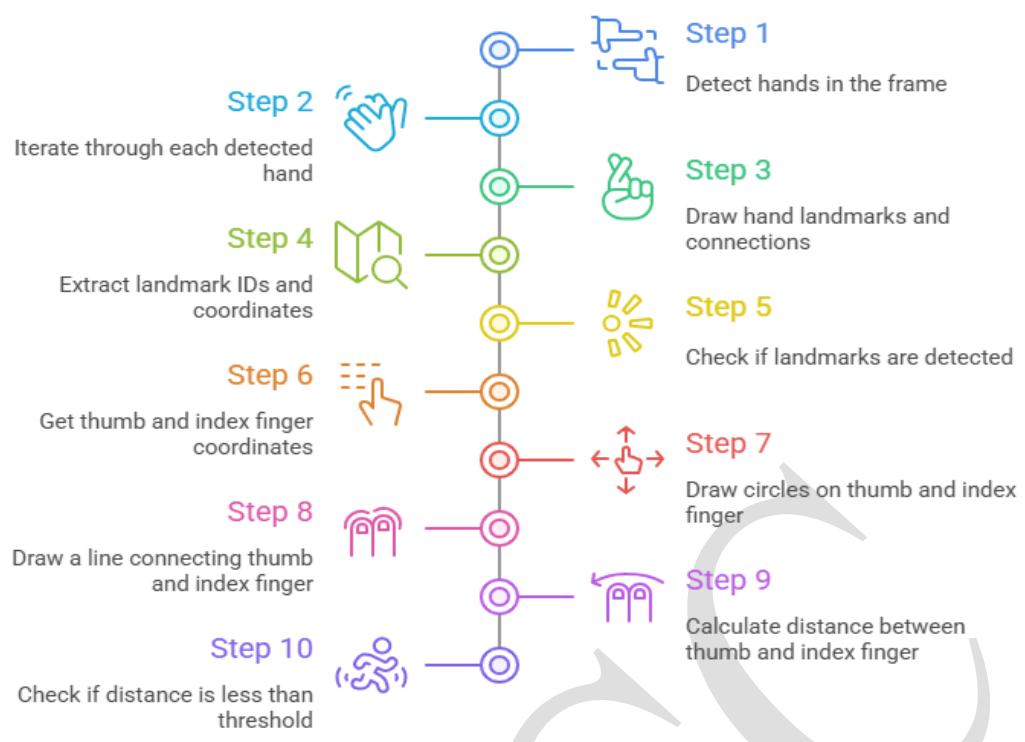
Fig 8. Step by Step Approach for Real-Time Hand Gesture Volume Control System
